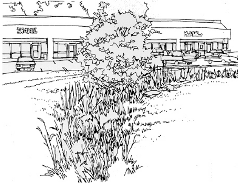
Figure II.A.2.(e). Biofiltration swales can incorporate storm water management in a soft, attractive, naturalistic way. At this shopping center, a drainage swale in a central open space serves as a visual amenity.
