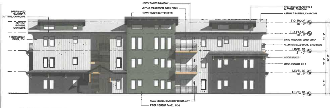
1 BUILDING A - EAST ELEVATION 1/8" = 1'-0"
