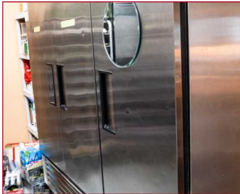
Commercial refrigerators and freezers
