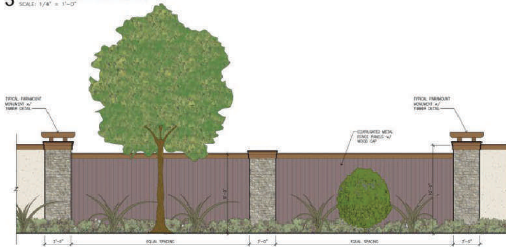
4 PERIMETER FENCE DETAIL #1 SCALE: 1/4" = 1'-0"
