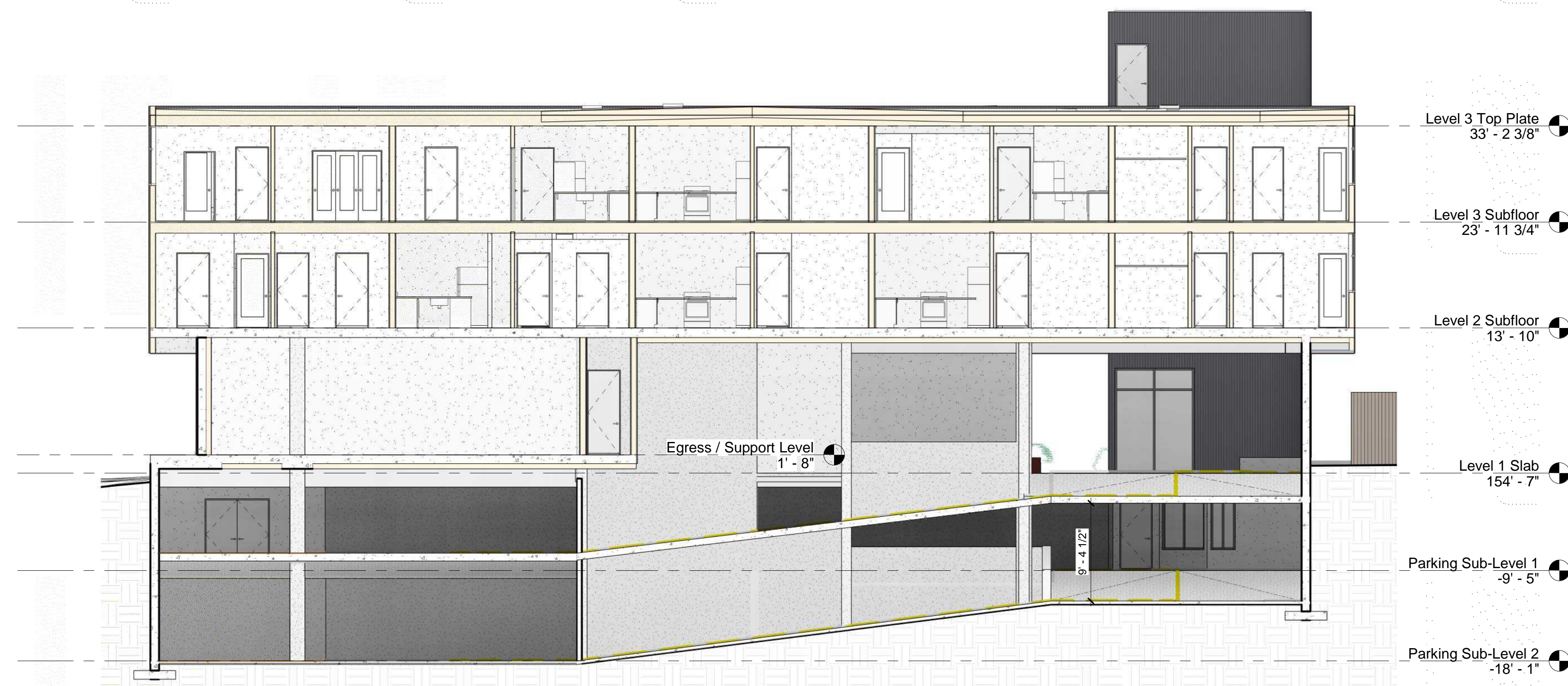
① N-S Through Garage Ramps 1/8" = 1'-0"
