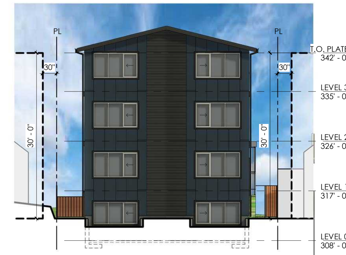
SDR - WEST ELEVATION SCALE: 3/32" = 1'-0"
