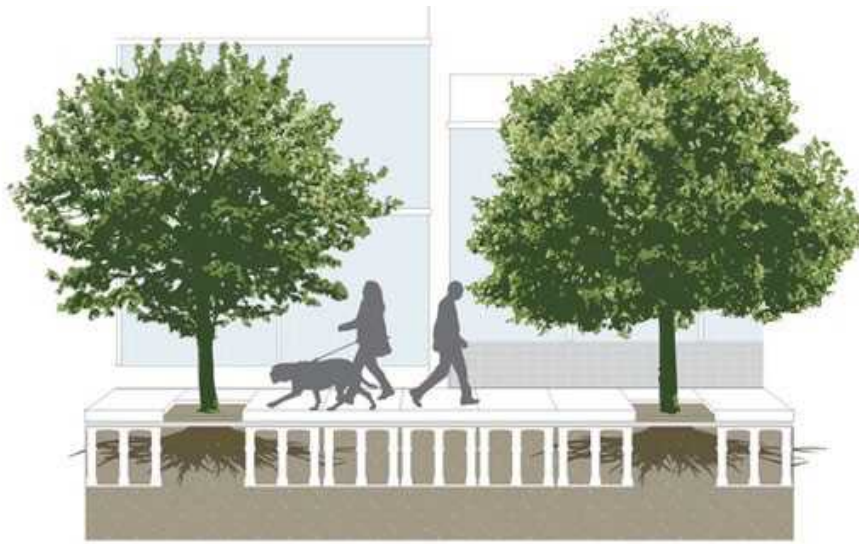
Image: Suspended pavement system.
