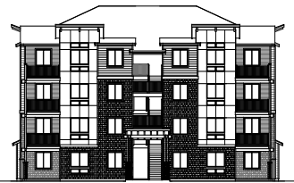
BUILDING 2 3/32" = 1'-0" FRONT/REAR ELEVATION
